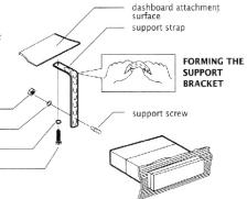
Bend the backstrap to conform to the mounting case and the dashboard surface to which you plan to secure the backstrap. Slide one of the utility holes on the backstrap onto the support screw and fasten it with the spring washer and nut provided.
